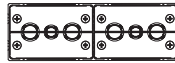
T6-LB-UN Allows mounting of 4 IPS inserts or six cables. Can also be used to block off a section
