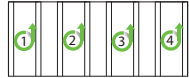
RT6-R-LB-RTMKT RT6-S-LB-RTMKT Mounting kits for using up to four FSR TBRT retractors in "R" or "S" style boxes. See LIT1497 TBRT Retractor Spec for details.
