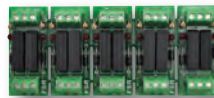
Adds relay control capability to FLEX systems for automated window treatments, lighting, etc.
