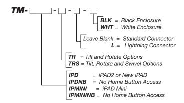
Example: A TM-IPDNB-TRS-L-WHT would be a TM-IPD desk mount for an iPAD2 or new iPAD with No Home Button Access, Rotate, Tilt and Swivel mechanics and Lightning Connector in White.
