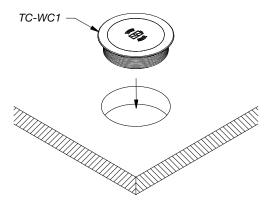
3. SECURE TC-WC1 WITH COLLAR. USE INCLUDED SPANNING TOOL TO SECURE TIGHTLY.
