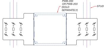
THE PWB-20X-MNT IS A SET OF BRACKET EARS THAT ALLOW THE INSTALLER TO POSITION THE PWB-200 OR PWB-203 AT DIFFERENT LOCATIONS BETWEEN THE STUDS WHILE MOUNTING.
