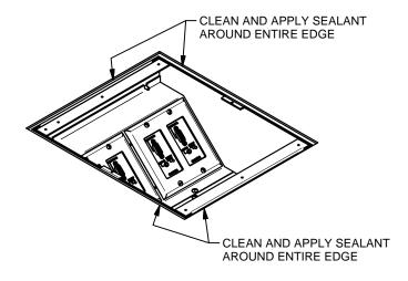
3. INSTALL COVER WITH SUPPLIED O-RINGS AND FLAT HEAD SCREWS. INSTALL FINISHED FLOORING MATERIAL.
