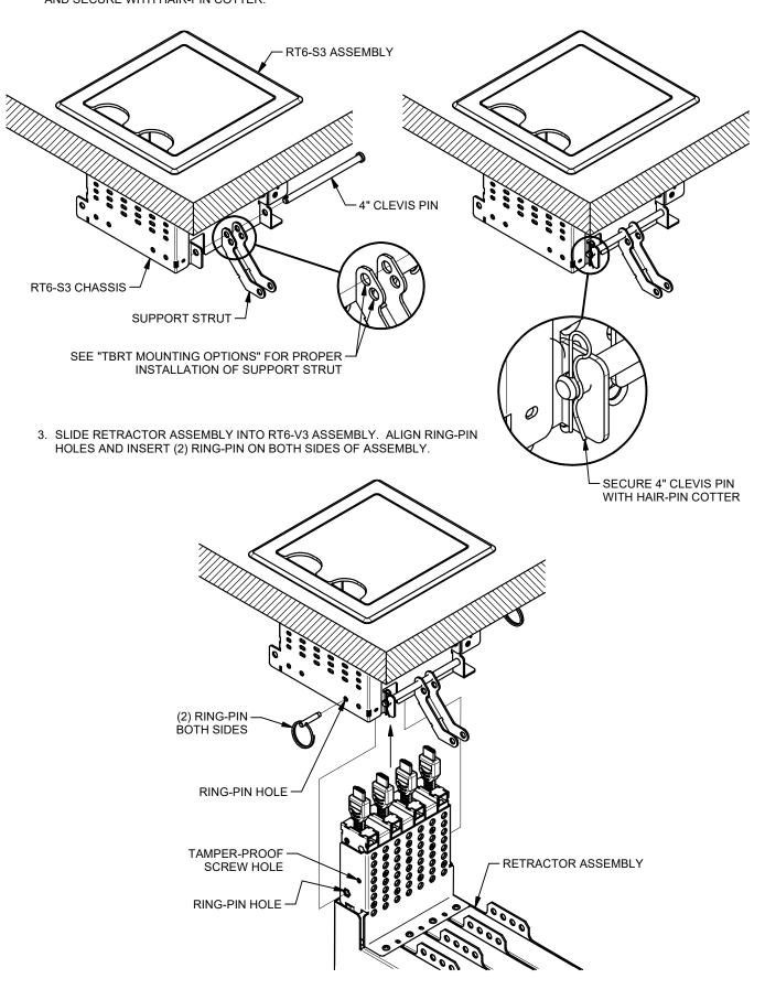
4. ALIGN SUPPORT STRUT HOLE WITH RETRACTOR FLANGE HOLES AND INSERT APPROPRIATE-LENGTH CLEVIS PIN. SECURE CLEVIS PIN WITH HAIR-PIN COTTER. FOR ADDITIONAL TAMPER-PROOF INSTALLATION, INSTALL (2) #6-32 x 1/4 LONG PAN HEAD SCREW.
