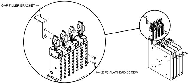
1c. INSTALL CHASSIS SUPPORT BRACKET. 1 REQUIRED FOR 1 RETRACTOR INSTALLED. FOR 2-4 RETRACTORS SUPPORT BRACKET IS OPTIONAL.
