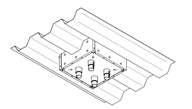
9. PULL WIRES AND CABLES TO BOX AS NECESSARY (CONFIGURING OF GANG MOUNTING BRACKETS MAY BE REQUIRED - REFER TO FLOOR BOX INSTALLATION INSTRUCTIONS). TERMINATE WIRES AND CABLES TO ELECTRONIC COMPONENTS, AND INSTALL ELECTRONIC COMPONENTS ONTO GANG MOUNTING BRACKETS. REINSTALL TEMPORARY COVER IF FINISHED COVER IS TO BE INSTALLED AT A LATER DATE.
