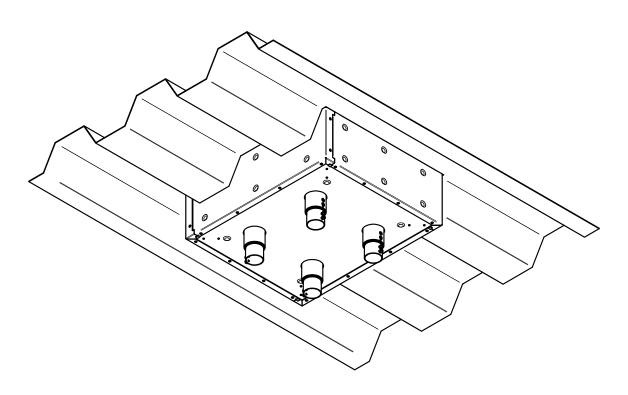
9. PULL WIRES AND CABLES TO BOX AS NECESSARY (CONFIGURING OF GANG MOUNTING BRACKETS MAY BE REQUIRED - REFER TO FLOOR BOX INSTALLATION INSTRUCTIONS). TERMINATE WIRES AND CABLES TO ELECTRONIC COMPONENTS, AND INSTALL ELECTRONIC COMPONENTS ONTO GANG MOUNTING BRACKETS. REINSTALL TEMPORARY COVER IF FINISHED COVER IS TO BE INSTALLED AT A LATER DATE.
