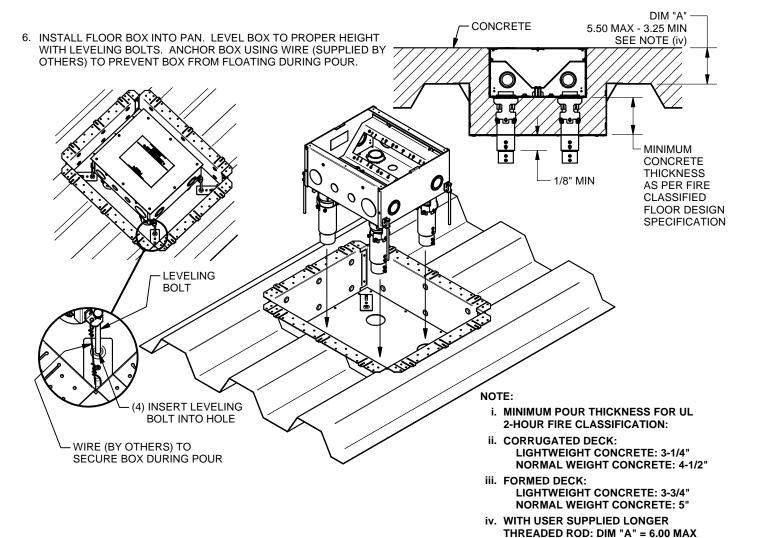
7. GANG BRACKET SCREWS AND GROUND SCREWS MUST BE IN PLACE AND BOTTOMED TO ENSURE SCREW VOIDS AFTER POUR. REINSTALL TEMPORARY COVER. FILL VOIDS BETWEEN DECK CUT-OUT HOLE AND PAN WITH TAPE OR CAULK TO PREVENT CONCRETE LEAKAGE WHILE POURING. DURING POUR, A VIBRATORY TOOL MUST BE USED TO ENSURE COMPLETE FILL OF CONCRETE SURROUNDING THE
