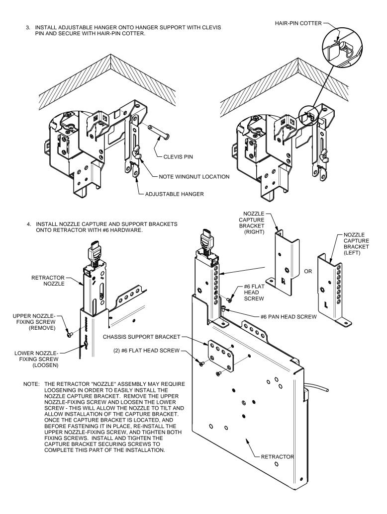
5. SLIDE RETRACTOR ASSEMBLY UP INTO T3-IPS ASSEMBLY.
