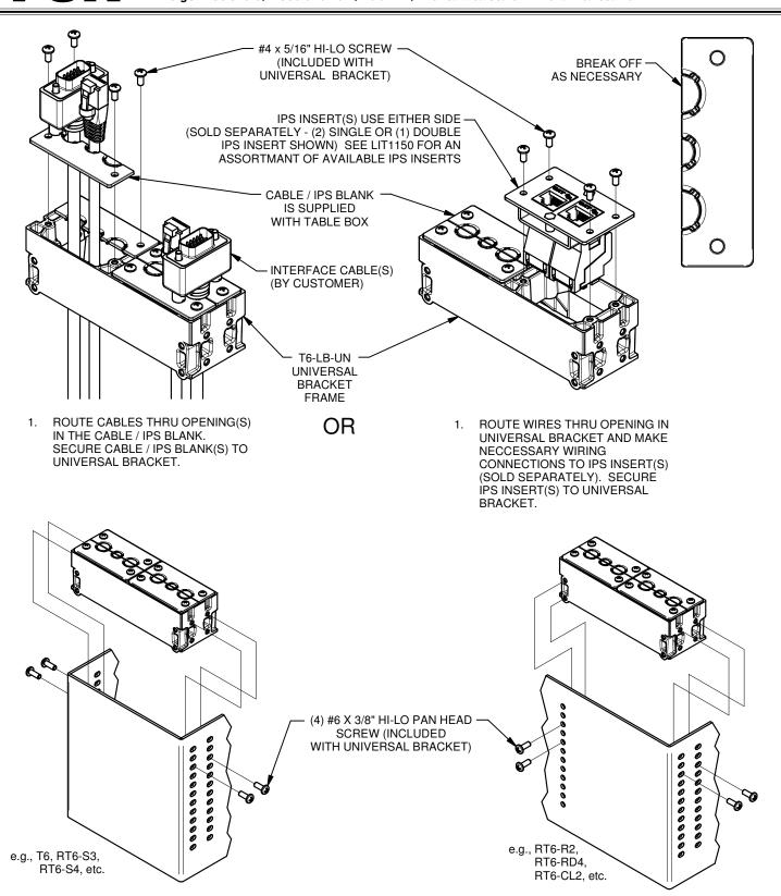
2. DETERMINE MOUNTING HEIGHT AND INSTALL UNIVERSAL BRACKET INTO CHASSIS. UNIVERSAL BRACKET MAY BE INSTALLED FROM TOP OR BOTTOM.
