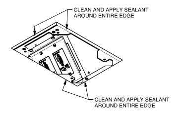
3. INSTALL SF4 ADAPTER PLATE WITH SUPPLIED FLAT HEAD SCREWS. APPLY RTV SILICONE SEALANT TO UNDERSIDE OF SCREWS. REFER TO SF4 COVER INSTALLATION INSTRUCTIONS TO COMPLETE INSTALLATION.
