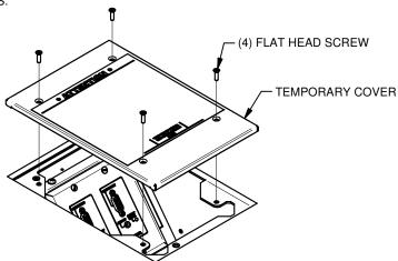
2. INSTALL CABLE INTERFACES AND CONNECTOR PLATES IF PREVIOUSLY NOT INSTALLED. CLEAN AREA IN AND AROUND ENTIRE TOP EDGE OF BOX AND APPLY 1/4" CONTINUOUS BEAD OF RTV SILICONE SEALANT.
