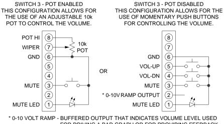
FOR DRIVING A BAR GRAPH OR FOR PROVIDING FEEDBACK TO A CONTROL SYSTEM DESIGNED TO DRIVE A 10k ohm LOAD.
