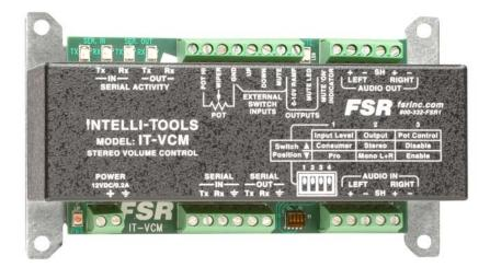
ASCII or Hardwire Controlled Line Level Volume Control Module with Serial Loop Through
