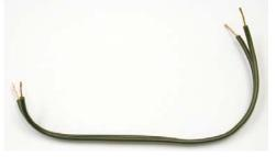
Step 2. Strip insulation back 3/16" from the end of the cables
