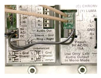
Step 5. Screw down the connections and tug on them to check for loose cables.
