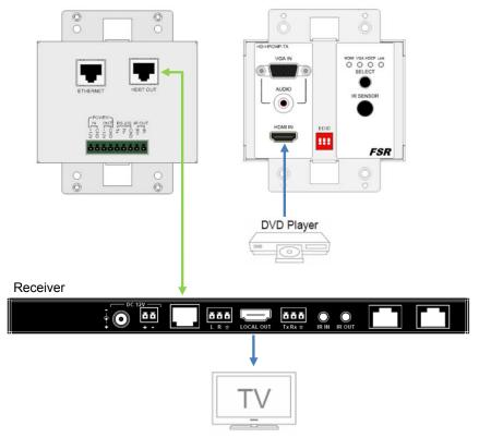
**NOTE:** Only one power supply is needed to power the Transmitter and Receiver set from any of the FSR's 100m HDBaseT receivers. The HD-HPCWP-Tx transmitter can be powered locally but it cannot send power to the receiver. Transmitters do not include a Power Supply. An FSR 17762 Power Supply is included with any of the FSR HDBaseT Receivers. FSR 17762 Power Supplies can also be ordered separately.
