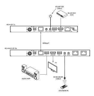
The HD-H-SP-Tx Transmitter is shown in the illustrations throughout this manual. Please note that any of the FSR 100m HD transmitters may be used with the HD-HAUD-SP-Rx Receiver.
