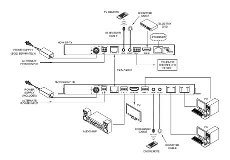
NOTE: Transmitters do not include a Power Supply. An FSR 17762 Power Supply is included with any of the FSR HDBaseT Receivers. Only one power supply is needed to power the Transmitter and Receiver set. FSR 17762 Power Supplies can also be ordered separately.
