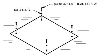
4. SECURE COVER TO BOX; SLIP PROVIDED O-RINGS ONTO PROVIDED 1"-LONG SCREWS, RIGHT UP TO THE SCREW'S HEAD, AND TIGHTEN THESE SCREWS INTO THE COUNTERSUNK THROUGH-HOLES.
