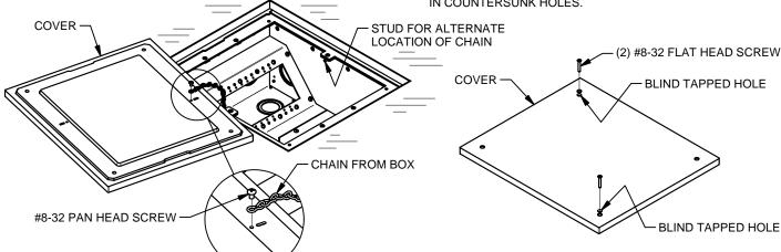
2. INSTALL BOX-ATTACHED CHAIN TO COVER WITH PROVIDED  $\#8-32 \times 1/4$ " PAN HEAD PHILIPS SCREW. CHAIN FROM BOX CAN BE REMOVED AND INSTALLED IN ALTERNATE LOCATION, IF DESIRED.
