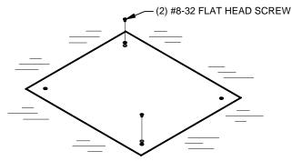
5. INSTALL PROVIDED #8-32 x 1/4" FLAT HEAD PHILIPS SCREWS INTO BLIND TAPPED HOLES ON COVER.
