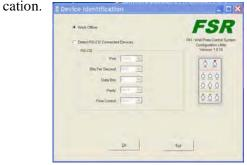
Select "Detect RS-232 C onnected Devices", leave the default comm settings except make sure the Port is correct for your computer and click the "Ok" button. The CU will establish communication with the connected RN-WPCS and the main application
