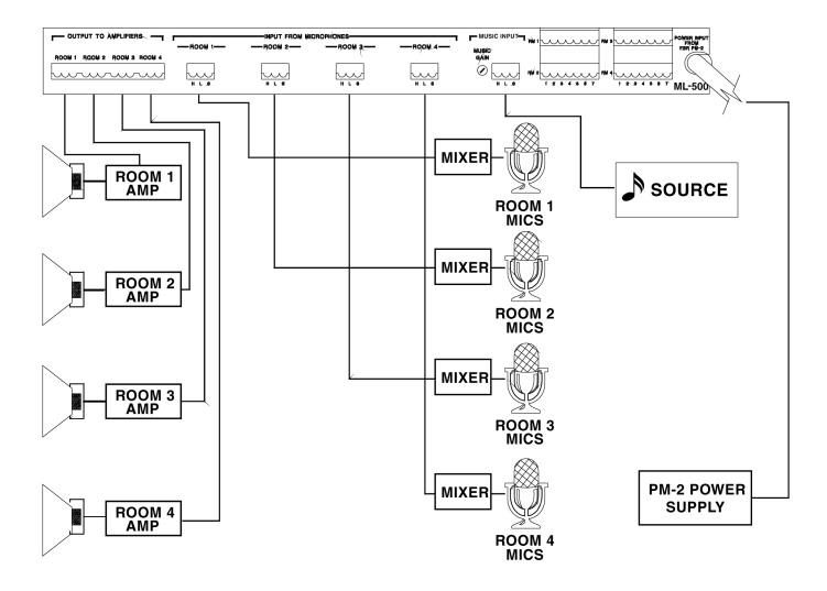
The microphone and music inputs are three pin screw terminals and can be wired one of two ways:
