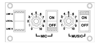
Have someone talk into each room's microphone in turn and adjust each room's mixer output level for a comfortable listening level (this means the same level as agreed upon when setting up the music) in each room.
