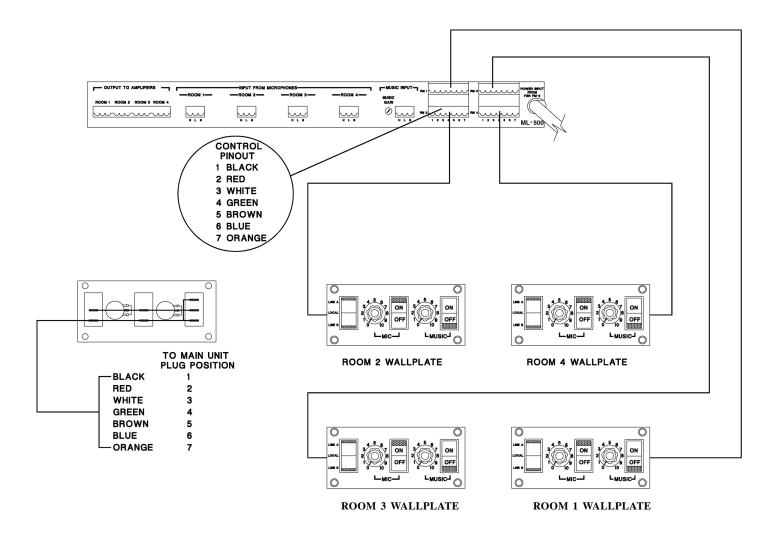
NOTE: Use the insulated self piercing connectors to connect the wallplate wires to the already installed cable (West Penn #271). To use these splicing connectors just insert the wallplate wire and the corresponding cable wire and crimp with a pair of plier
