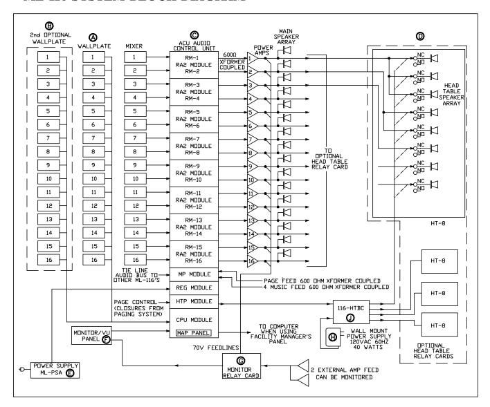
A....... There are two types of wallplates available for use in the ML-116 system, membrane and LCD. Both control all wallplate functions. These functions include Music Selection, Room Mixer Enable, Music Enable and Volume, and Local Input On/Off and Volume.
