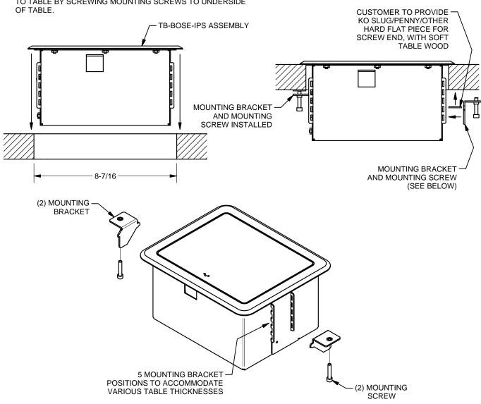
4. INSTALL IPS PANELS (SOLD SEPERATELY) AND MAKE ELECTRICAL CONNECTIONS AS REQUIRED.
