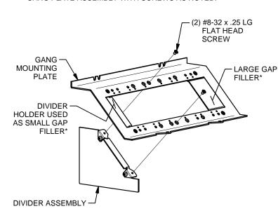
\* GAP FILLERS ARE OPTIONAL, PER DESIRED CONFIGURATION (SEE PREVIOUS PAGE). AND ARE INSTALLED SIMILARLY TO DIVIDER ASSEMBLIES
