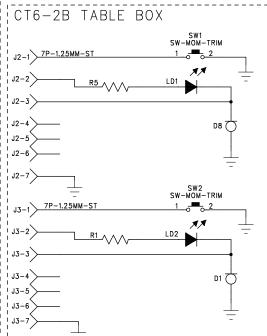
Led Current: internally regulated at 16 mA nominal over recommended operating voltage range.
