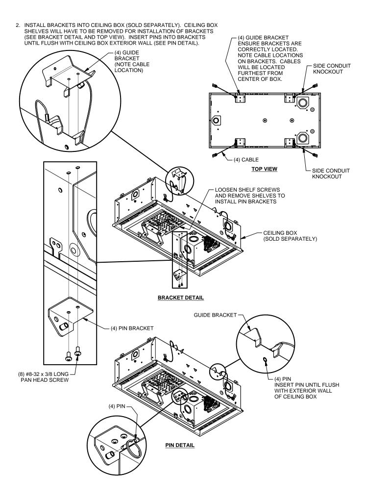
3. ALIGN THE CEILING BOX, WITH ITS NEW BRACKETS, WITH THE CAPTURE BRACKETS INSIDE FRAME. ATTACH 2 CABLES FROM CEILING BOX (NEAREST THE BOX'S KO'S) TO FRAME AND ROUTE WIRING INTO CEILING BOX.
