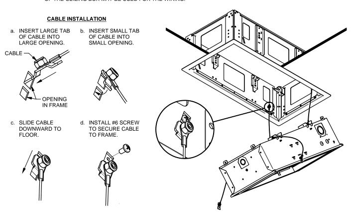
4. AFTER ALL WIRING IS ROUTED TO CEILING BOX, ATTACH REMAINING CABLES TO FRAME.
