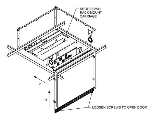
4. REMOVE #8-32 SCREW AS SHOWN, AND REMOVE OUTLET GRILL. SUPPORT OUTLET GRILL WHILE REMOVING SCREW. INSTALL FAN KIT PER INSTRUCTIONS. RE-INSTALL OUTLET GRILL AND CEILING BOX DOOR BACK INTO CEILING BOX BY REVERSING THEIR REMOVAL STEPS.
