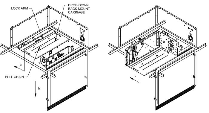
6. INSTALL WIRE BUNDLE INLET, WIRE INLET FOAM, AND WIRE INLET COVER TO SIDES OF BOX. REMOVE THE FOAM BLOCKS NECESSARY FOR THE WIRE BUNDLE EXITING THE BOX. PULL WIRES TO CEILING BOX THRU WIRE INLET OR CONDUIT AS REQUIRED.
