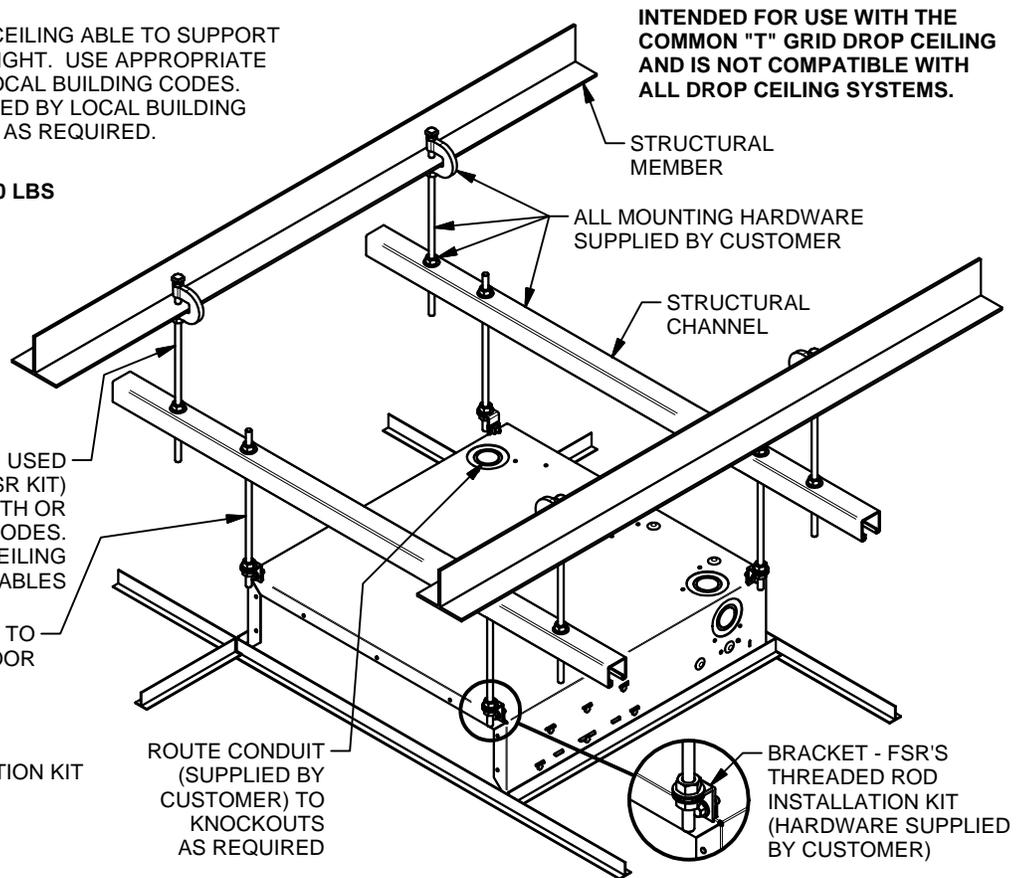
**INTENDED FOR USE WITH THE COMMON "T" GRID DROP CEILING AND IS NOT COMPATIBLE WITH ALL DROP CEILING SYSTEMS.**
