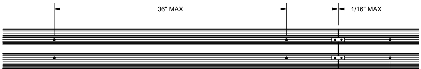
MINIMUM SCREW PATTERN ON TOP OF CARPET
