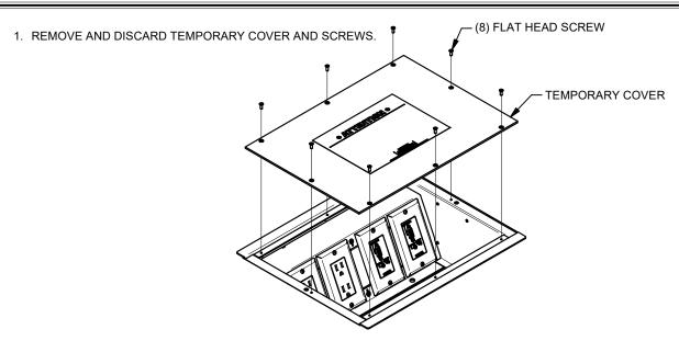
2. INSTALL ELECTRICAL DEVICES AND CONNECTOR PLATES IF PREVIOUSLY NOT INSTALLED.
