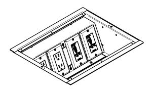
3. INSTALL COVER WITH SUPPLIED FLAT HEAD SCREWS.
