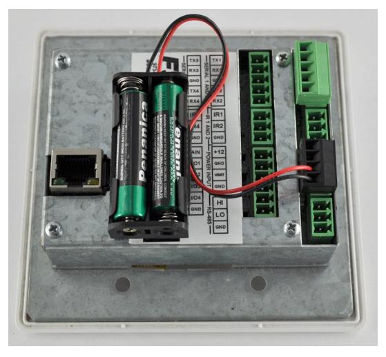
Peel off the double sided tape and attach the battery holder as shown, then install the batteries and wires to VBAT(Red wire) and GND(Black wire) terminals..
