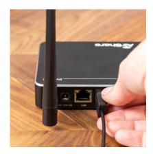
5) Connect an HDMI cable to the HDMI input (ID 7). Proceed to number 7 if no secondary source is being used in application
