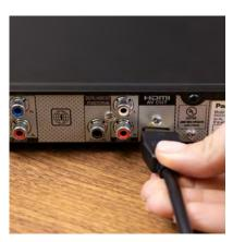
7) HDMI Output (ID 5): Connect an HDMI cable from this port to an HD display.
