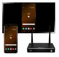
**Step 9:** On the mobile device, swipe down on the main screen and tap the mirroring button to the "off" position to stop mirroring.
