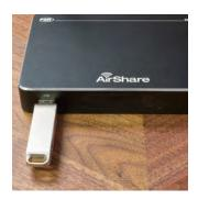
**Step 2:** Remove WMT-MINI from AirShare and plug into PC/Laptop
