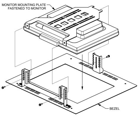
ADJUST THE LOCATION OF THE MONITOR'S VIEWING SCREEN SO THAT IT'S CENTERED IN THE OPENING IN THE BEZEL, AND CHECK THIS ADJUSTMENT BY FLIPPING THE ASSEMBLY UP OR OVER, UNTIL PROPER SCREEN LOCATION IS ACHIEVED. TIGHTEN ALL FOUR MONITOR SCREWS TO MAINTAIN IT'S POSITION. 43031
