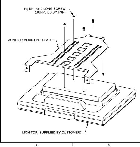
REINSTALL MONITOR MOUNTING PLATE (WITH MONITOR) ONTO BEZEL ASSEMBLY, ENSURING THE MONITOR'S OUTER RIM RESTS, ALL AROUND, ON BEZEL'S REAR SURFACE. MAINTAIN THIS POSITION BY COMPLETELY TIGHTENING ORIGINAL HEX-HEAD SCREWS.
