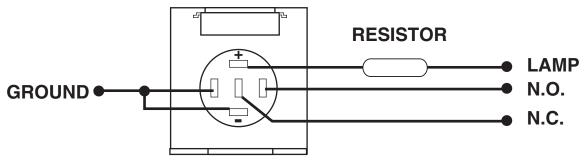
THE LED IN THE SWITCH ASSEMBLY IS RATED AT 20 ma. IF THE DEVICE DRIVING THE LED IS CURRENT LIMITED TO 20 ma OR LESS, THE SERIES RESISTOR IS NOT REQUIRED.
