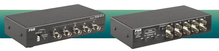
The RGB-HV-2 is an ultra high resolution, ultra high bandwidth 1x2 distribution amplifier for applications requiring the highest possible video quality. Each of the 2 output stages has independent cable equalization to compensate for variations in the cable's response.
