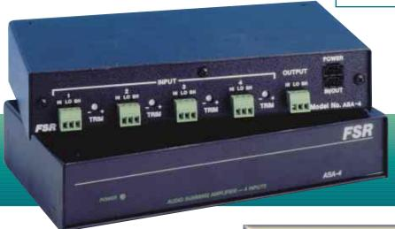
The ASA-4, audio summer, will sum or mix up to 4 line level inputs and provides one transformer coupled line level audio signal output. The ASA-4 features unity gain which means no input signal is attenuated as happens in any passive mixing device. The residual noise (<80 db) insures that the fidelity of the incoming signals is not compromised in any way. The transformer coupling of the output insures that ground loop problems are completely eliminated.
