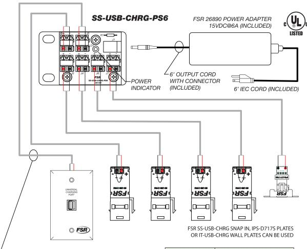
TWO CONDUCTOR HOOK-UP WIRE (INSTALLER PROVIDED). TWO OHM MAXIMUM ROUND TRIP. SEE CHART FOR LENGTH VS. GAUGE REQUIREMENTS.
