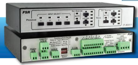
The IT-AS411 Series Audio Switchers are 4x1 audio switchers that have an extra mic/line level input for a voice lift system or direct microphone input. All models have four switched program audio inputs and an independent mic or line level input that is summed (mixed) with the selected active program audio.
