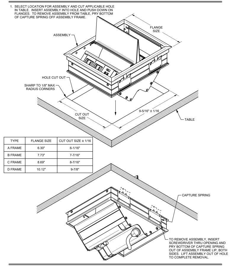
43347 LIT1729A 2. IF APPLICABLE, INSTALL KEYSTONE CONNECTORS (SOLD SEPARATELY) INTO INSERTS (SINGLE OR DUAL), MAKE WIRING CONNECTIONS AS REQUIRED, AND INSTALL INSERTS INTO ASSEMBLY. IF KEYSTONE CONNECTORS ARE TO BE INSTALLED AT A LATER DATE INSTALL BLANK INSERTS. FRONT FACE MUST BE CLOSED WITH KEYSTONE OR BLANK INSERTS.
