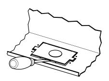
USE A SCREWDRIVER TO BREAK TABS ON BREAKOUT NEAREST BOX OPENING
