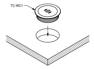
3. SECURE TC-WC1 WITH COLLAR. USE INCLUDED SPANNING TOOL TO SECURE TIGHTLY.
