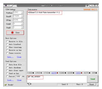
Type the commands in the data transmit window, for example "get sw\_version", click your PC **Enter** button and click the Uart Tool **Send** button, the Data receive window will show the response.
