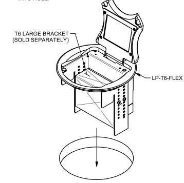
3. INSTALL BLANK OR SNAP-IN CONNECTOR (SOLD SEPARATELY) INTO UNDERTABLE MOUNTING BRACKET. INSTALL APPROPRIATE-LENGTH #6-32 THREADED RODS INTO LP-T6-FLEX. SECURE UNDERTABLE MOUNTING BRACKET WITH #6-32 LOCKING NYLON NUTS.
