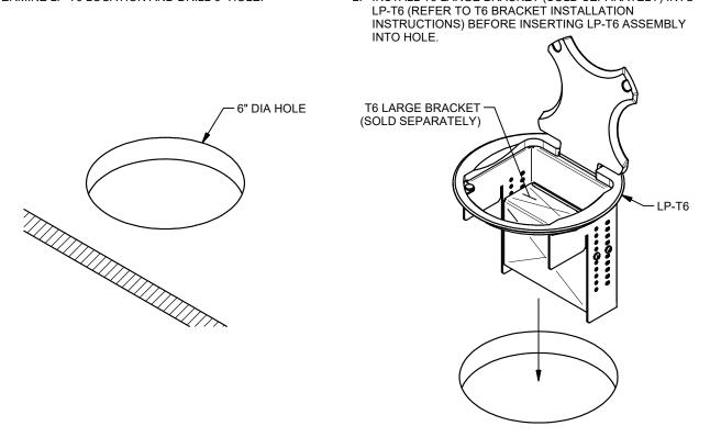
3. INSTALL BLANK OR SNAP-IN CONNECTOR (SOLD SEPARATELY) INTO UNDERTABLE MOUNTING BRACKET. INSTALL APPROPRIATE-LENGTH #6-32 THREADED RODS INTO LP-T6. SECURE UNDERTABLE MOUNTING BRACKET WITH #6-32 LOCKING NYLON NUTS.
