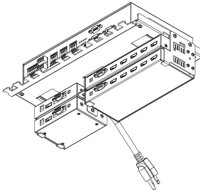
7. Thread the four 6-32 x 3/8" Pan Head Phillips screws into the 4 tapped holes on the under table controller bracket but do not tighten. (The Control Chassis will be mounted (hung) from these screws in the next step.)
