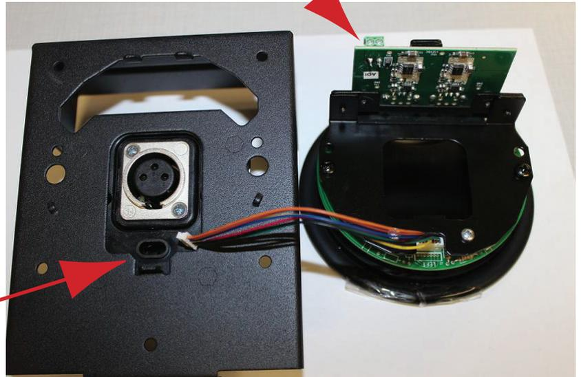
After installing the under table lamp bracket, pass the power wire harness shown in picture through this hole.
