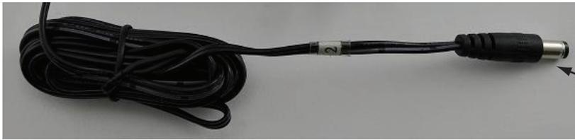
Cut the connector off of the supplied wallwart
