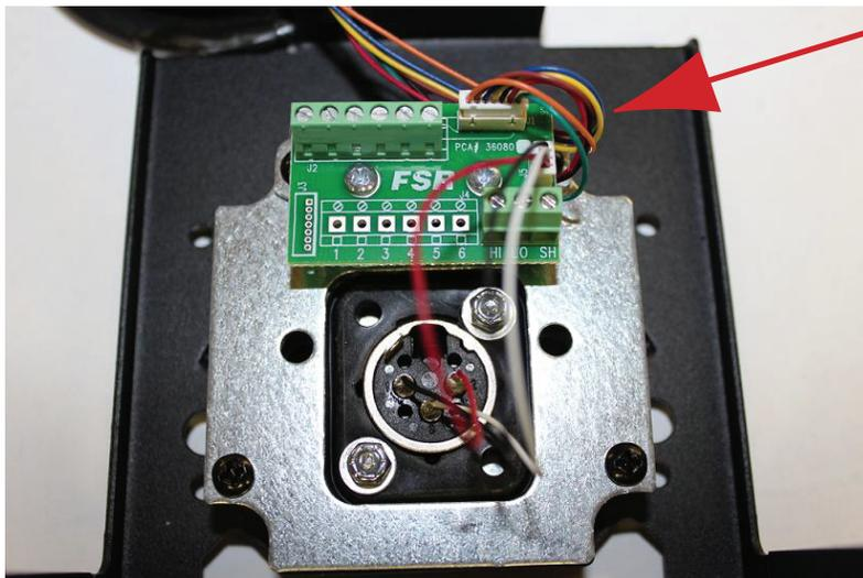
Pull the wire harness and plug as shown.
