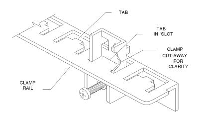
2. INSERT CLAMPS AS NEEDED INTO TOP AND BOTTOM CLAMP RAILS
