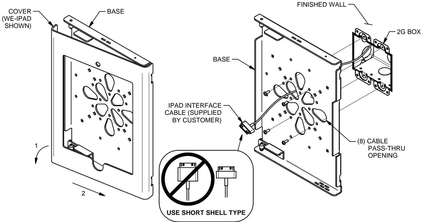
3. INSTALL PROVIDED SILICON SLEEVE TO IPAD (SUPPLIED BY CUSTOMER) AND MAKE ELECTRICAL CONNECTIONS AS REQUIRED. POSITION IPAD IN BASE AND SUPPORT IPAD FROM FALLING.
