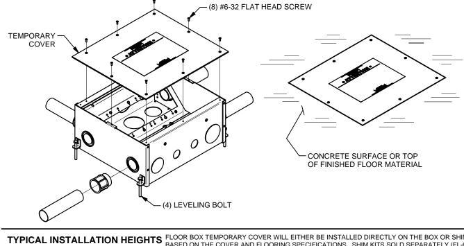
TYPICAL INSTALLATION HEIGHTS FLOOR BOX TEMPORARY COVER WILL EITHER BE INSTALLED DIRECTLY ON THE BOX OR SHIMMED BASED ON THE COVER AND FLOORING SPECIFICATIONS. SHIM KITS SOLD SEPARATELY (FL-600P-CSK). THE TEMPORARY COVER MAY NOT BE FLUSH WITH THE FINISH FLOOR IN ALL INSTALLATIONS. Carpeted or Tile Floors, Cover types - BLP, BSQ, B, SLP, SSQ, S
