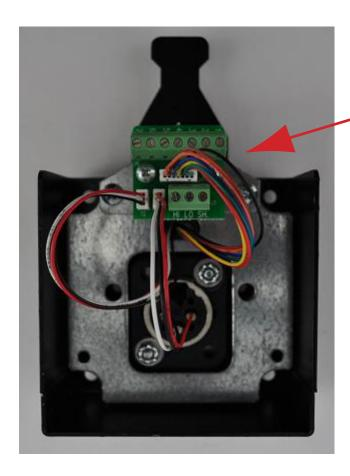
Plug the wire harnesses to PCB headers as shown.
