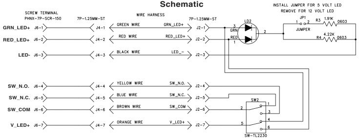
For Led drive use one or the other only: Connect to J6 Pin 1&2 for external led drive, or connect to J6 Pin 7 for self generated feedback.
