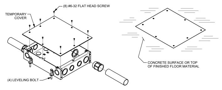
TYPICAL INSTALLATION HEIGHTS FLOOR BOX TEMPORARY COVER WILL EITHER BE INSTALLED DIRECTLY ON THE BOX OR SHIMMED BASED ON THE COVER AND FLOORING SPECIFICATIONS. SHIM KITS SOLD SEPARATELY (FL-500P-CSK). THE TEMPORARY COVER MAY NOT BE FLUSH WITH THE FINISH FLOOR IN ALL INSTALLATIONS.
